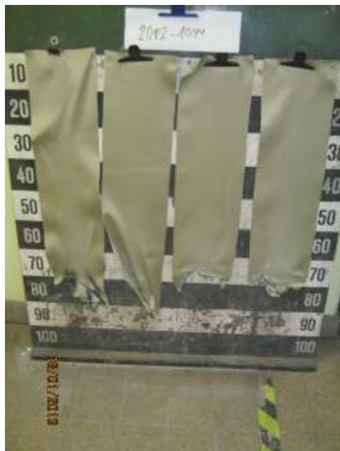
Appearance of the sample A after the "Brandschacht" test
