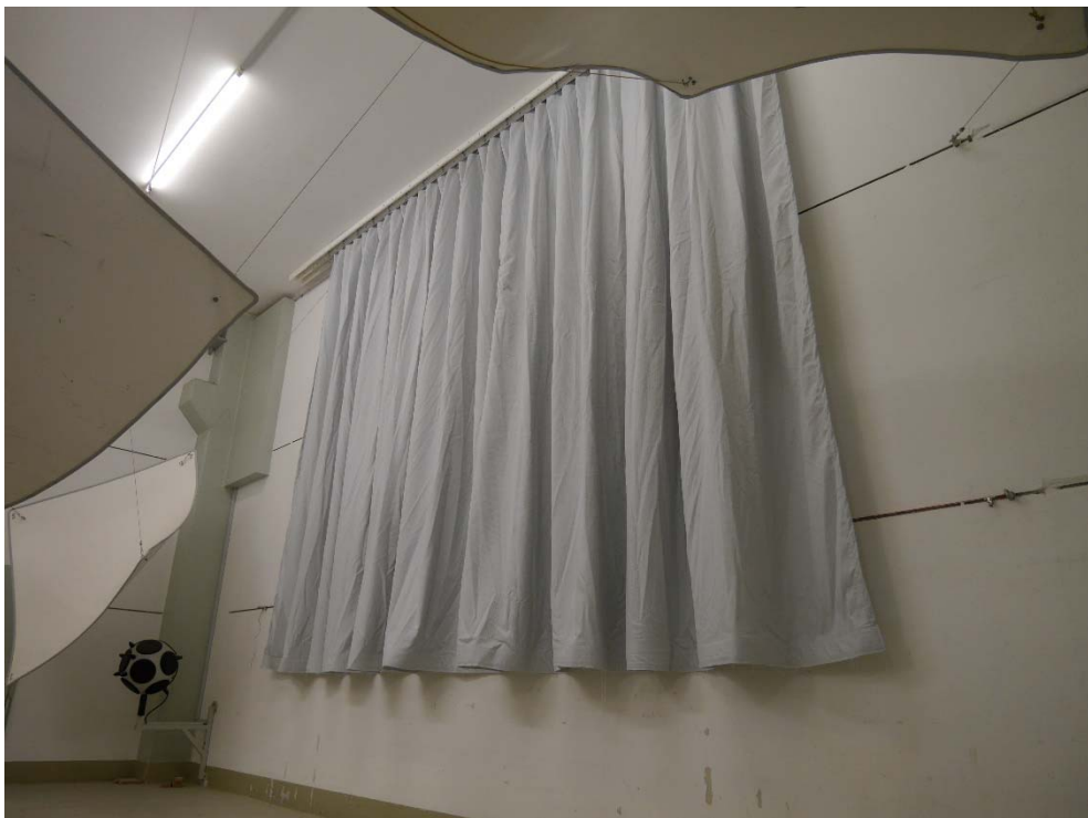
Figure B.4. Folded arrangement: test object mounted in the reverberation room, diagonal view.
