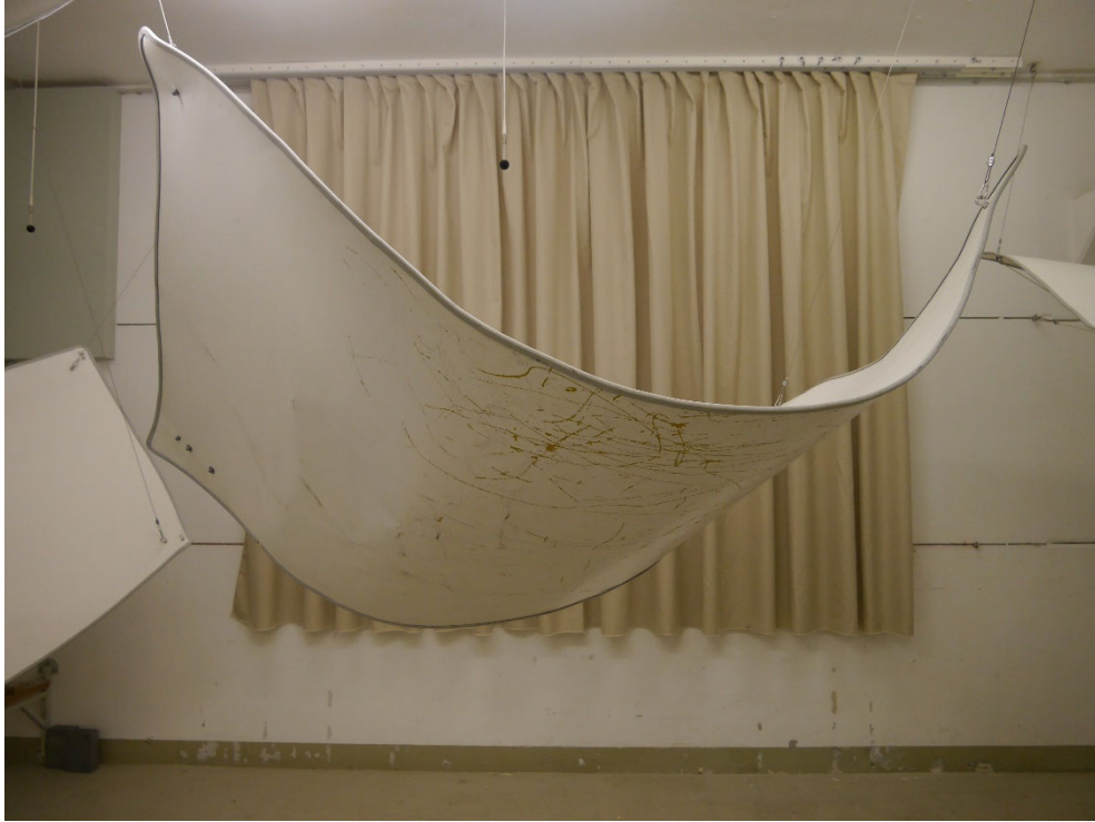
Figure B.3. Pleated curtain: test object mounted in the reverberation room, frontal view.
