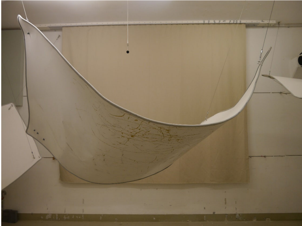
Figure B.1. Flat hanging curtain: test object mounted in the reverberation room, frontal view.
