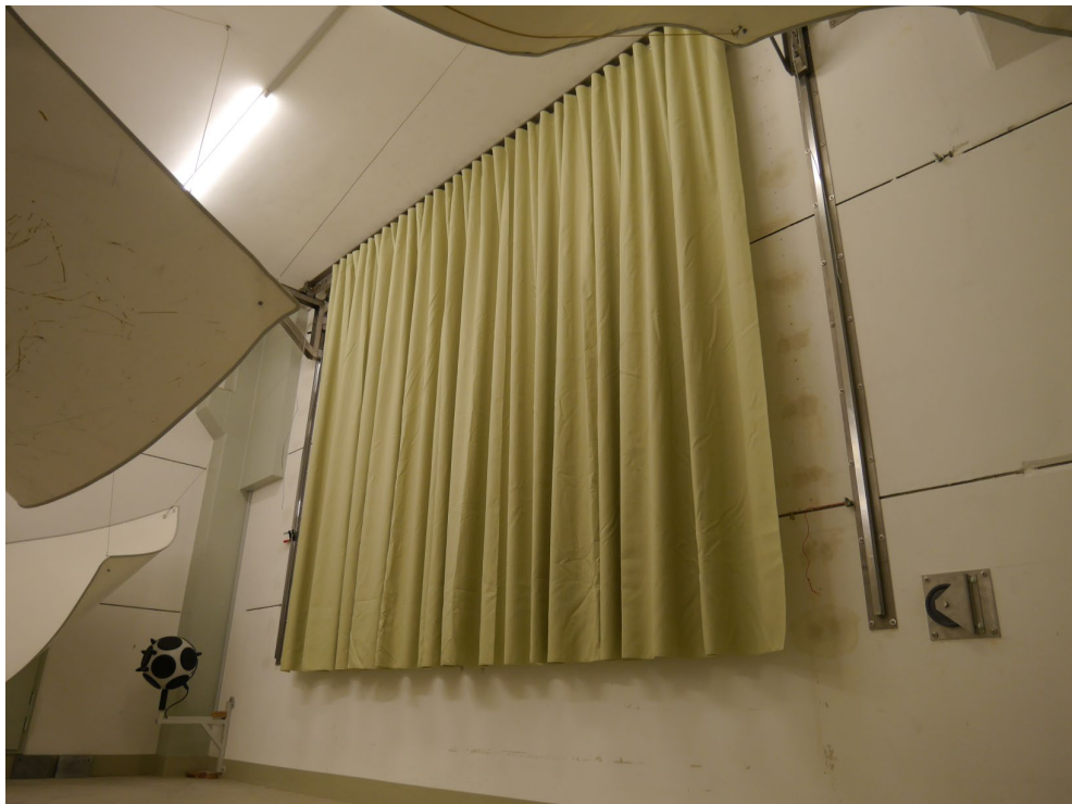
Figure B.4. Pleated curtain: test object mounted in the reverberation room, diagonal view.
