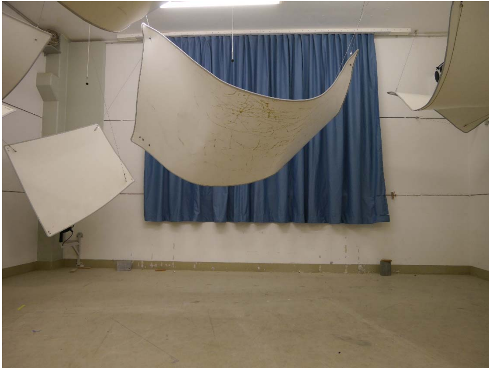
Figure B.3. Ruched curtain: test object mounted in the reverberation room, frontal view.
