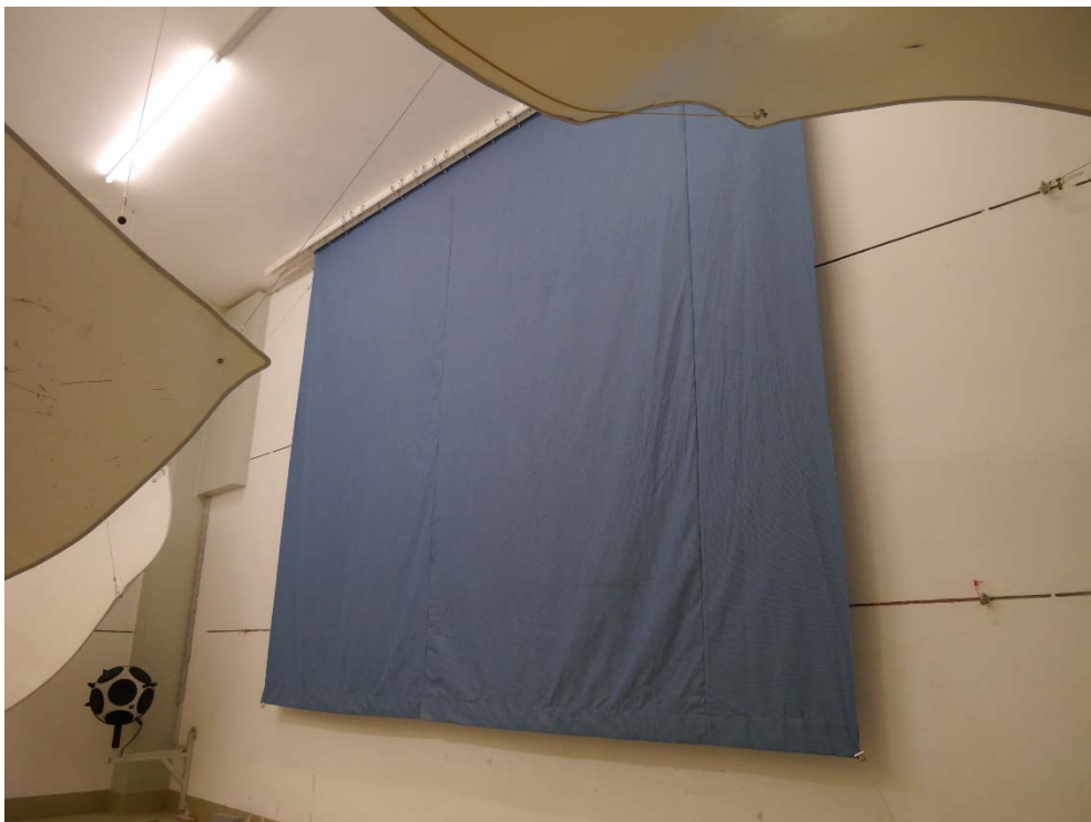
Figure B.2. Flat hanging curtain: test object mounted in the reverberation room, diagonal view.
