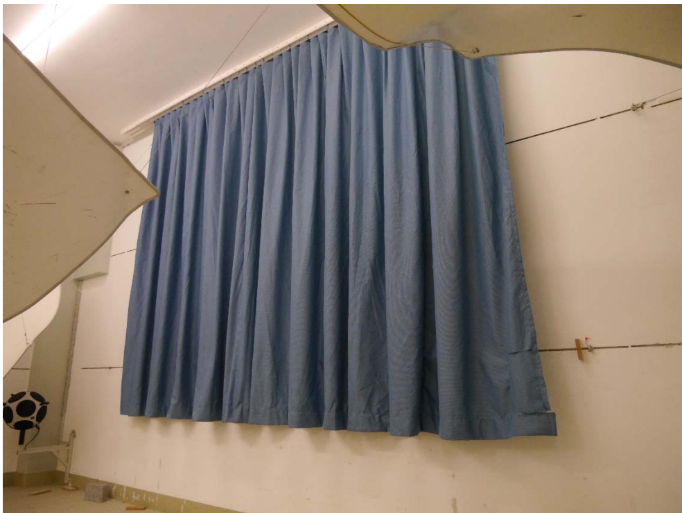
Figure B.4. Ruched curtain: test object mounted in the reverberation room, diagonal view.
